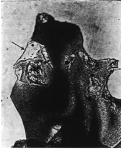
Figure 6. — Fragmentary thin slide of one of the sand fulgurites temporarily mounted in a liquid with n = 1.480 , showing on the left margin lechatelierite ( n = 1.457 ). The microscope tube is raised to show the Becke line. X 200.
