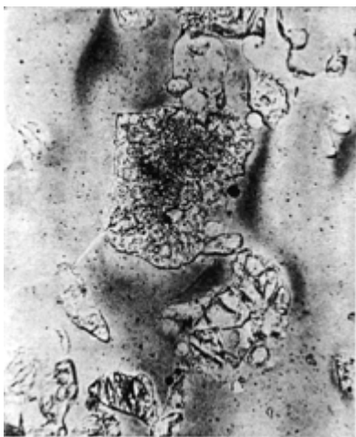
FIG. 8. — The large grain near the center has been altered on the exterior to cristobalite. The other grains are altered in part to lechatelierite. X 100.
