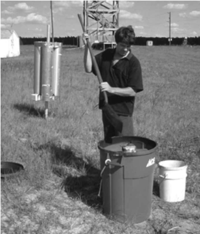
The rocket and the sand-filled receptacle used in McCollum's lightning-triggering experiment to create the fulgurite.
