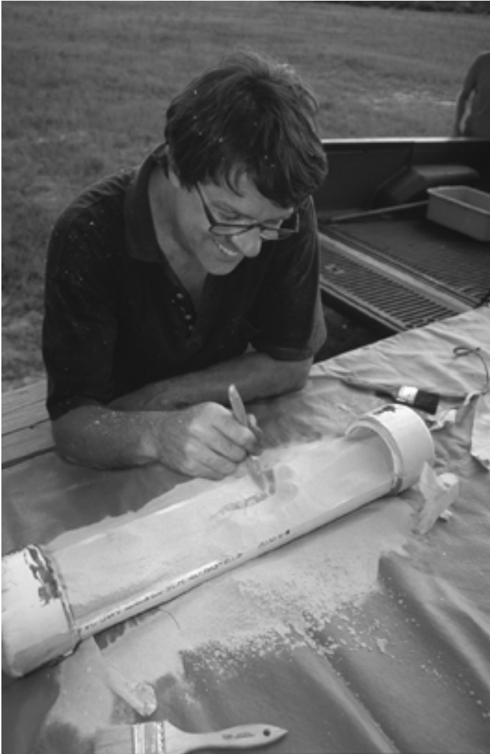
McCollum excavates his fulgurite from the PVC pipe “Pod” used as a receptacle for receiving the lightning strike at Camp Blanding.
