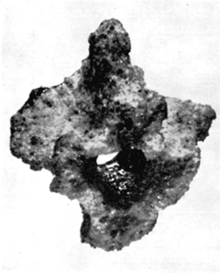
Figure 25: Oblique view of short piece of symmetrical end of specimen: a, looking through bore, and showing three complete ridges in perspective, and the four on the front face. Glassy surface of the bore indicated. X 4.
