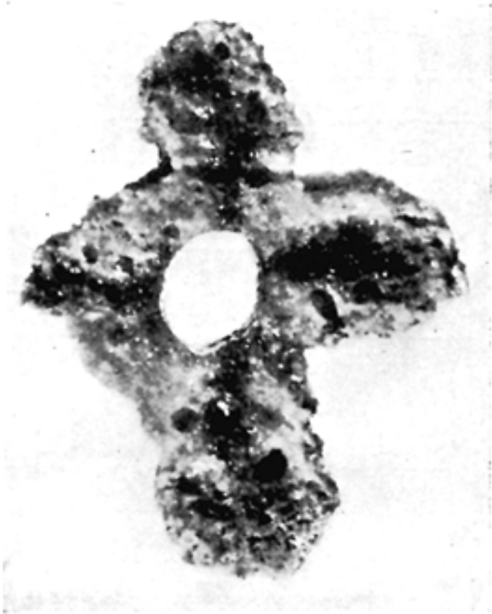
FIG. 26. Thick section of specimen A, showing the general form of a rectangular cross, and the dark colored bands in the middle plane of each ridge, lying in two right-angle planes. Some of the larger vesicles are prominent and smaller ones can be seen with magnification. Thin section of same shown in Fig. 30. X 4.
