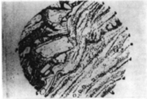
Figure 3: Microscopic photograph of rock fulgurite Magnification: x50
